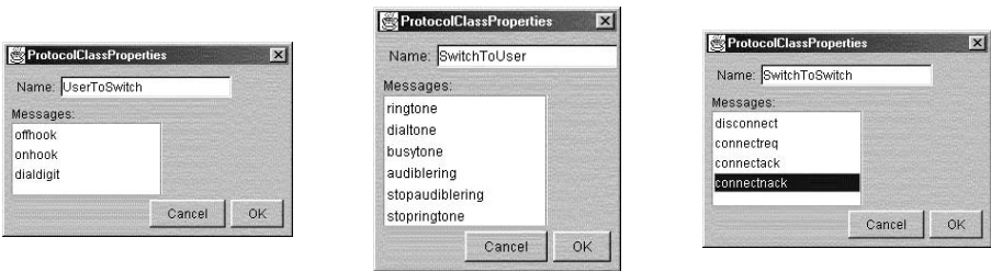
Fig. 5. Protocol class definition for POTS model.
